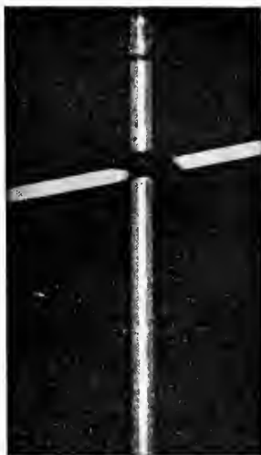
Fig. 26.— Polarization by double refraction of the dark rays emitted by bodies endowed with invisible phosphorescence. Duplication of one of the arms of the cross. The images are superposed at the central part, and allow us to compare the intensity of the duplicated parts (on the negative the central part is, of course, the darker).
