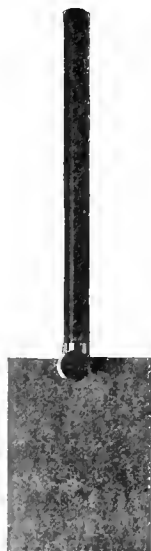
Fig. 6—Metal plate held by an insulating handle of ebonite. It can be brought to a potential of 1000 volts by rubbing it very slightly.
